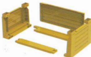
Embed the front bracket and rear bracket into side plate, put back plate into the transom. And repeat the above steps with other brackets.
