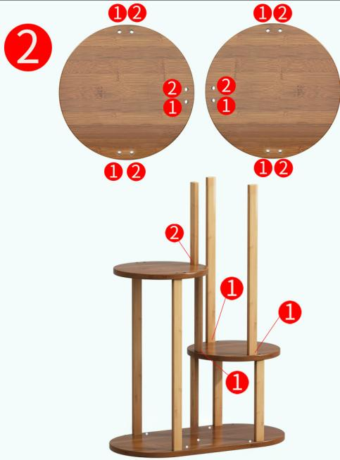
Install the 2nd and 3rd round shelves and poles. (Note: Align hole ① with ①, and ② with ②)
