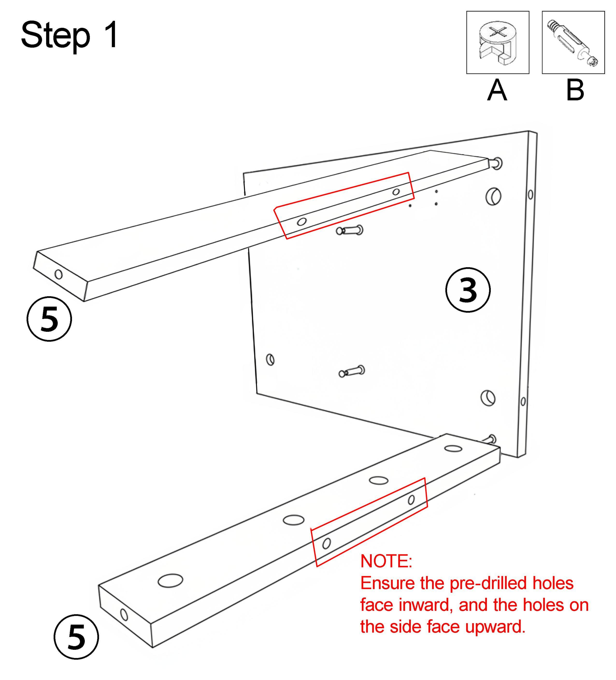
Install B into all white pre-installed holes on panel 3 and 5. Connect them and using A to lock.
