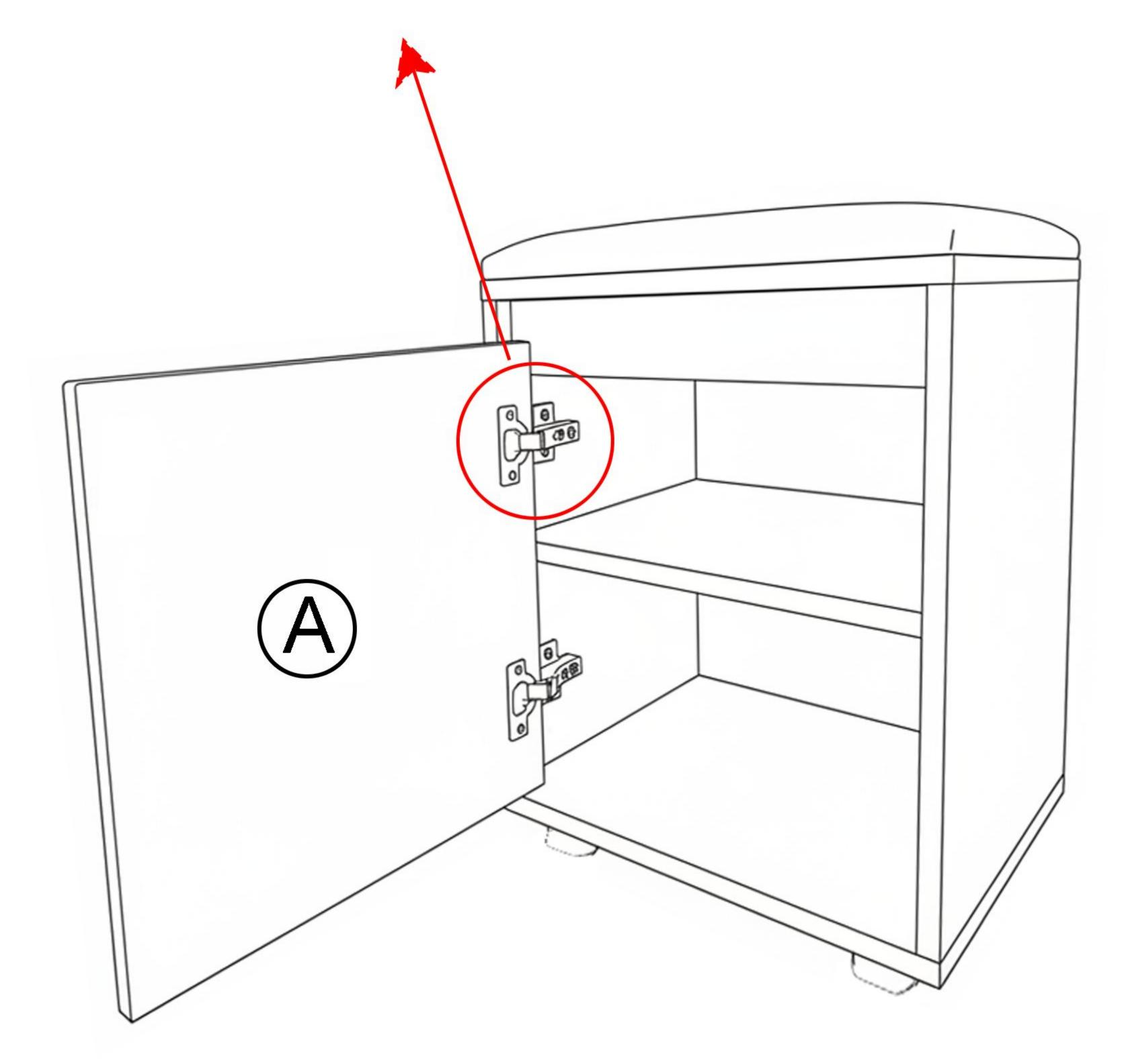
Align the hinge with the upper holes, fix it first, then install the lower hinge. If the lower holes are misaligned, adjust as needed. Refer to the initial hinge installation instructions to adjust the door's height and gap.
