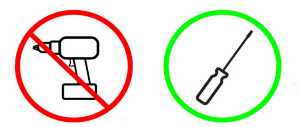
NOTE: Please be sure to use a manual screwdriver and refrain from using an electric drill.
