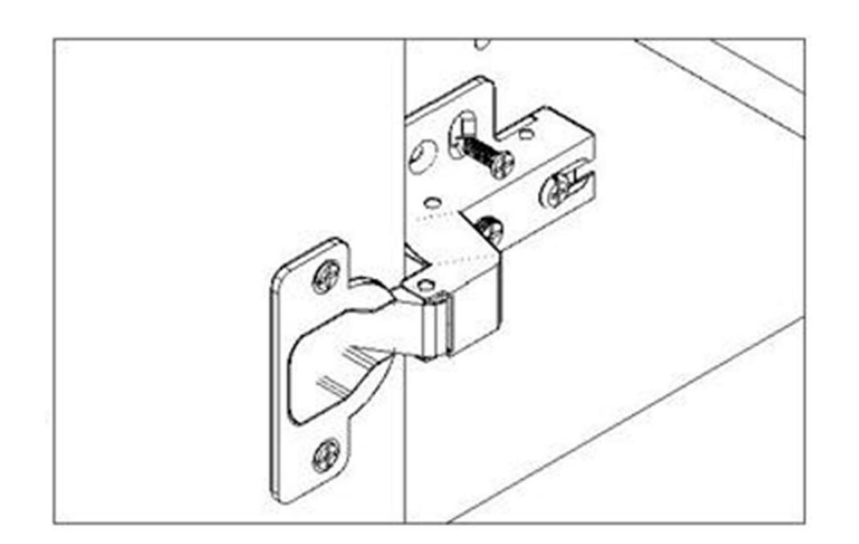
When installing the door panel, first secure the two rear holes of the hinge with C
